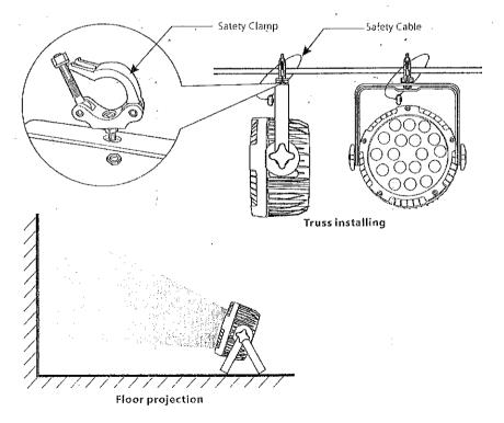
Regardless of the rigging option you choose for your FLATPAR 1818, always be sure to secure your fixture with a safety cable. The fixture provides a built-in rigging point for a safety cable on the hanging bracket as illustrated above. Be sure to only use the designated rigging point for the safety cable and never secure a safety cable to a carrying handle.
